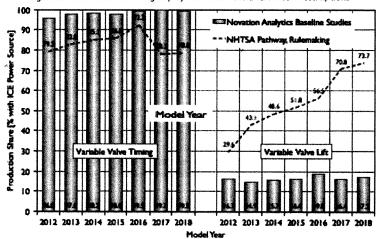
Figure 2: Variable Valve Timing Deployment Reol-World vs. NHTSA Assumptions
