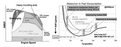
Figure X: Areas of cooled EGR usage for the Mazda CX-9 (left) and characterization of fuel consumption improvements at mid-range loads doe to cooled EGR (right). Both figures from Mazda.
