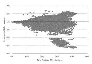
Figure 5 Incremental Effectiveness of 48V Mild Hybrid with belt-integrated starter-generator (BISG) to crankintegrated starter-generator (CISG) (Small Car class)
