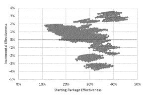
Figure 8 Incremental Effectiveness of the best six-speed (AT6L2) v. the best eight-speed (AT8L3) (Small SUV)
