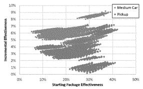
Figure 10 Incremental Effectiveness of six-speed (6AT) to eight-speed (8AT) for Pickup and Medium Car
