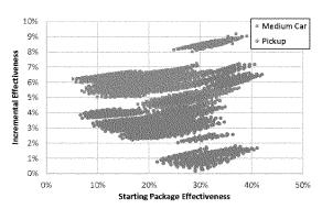
Figure 4 Incremental Effectiveness of six-speed (6AT) to eight-speed (8AT) for Pickup and Medium Car
