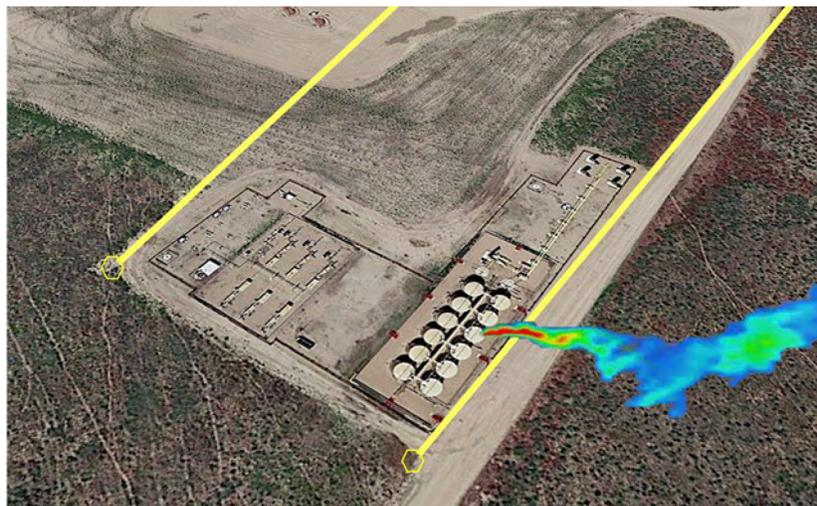
Laser beam paths (yellow lines) extend between the telescope (outside image top) to retroreflector locations (yellow hexagons), providing a fence bounding the monitored area. Sites are measured during wind conditions that favor high site coverage (potential plumes would cross bounding laser beams). A theoretical plume is shown emitting from the tanks and crossing the downwind beam.
