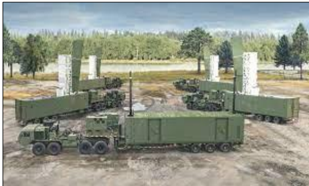
Figure 1. Typhon Launchers and Battery Operations Center
