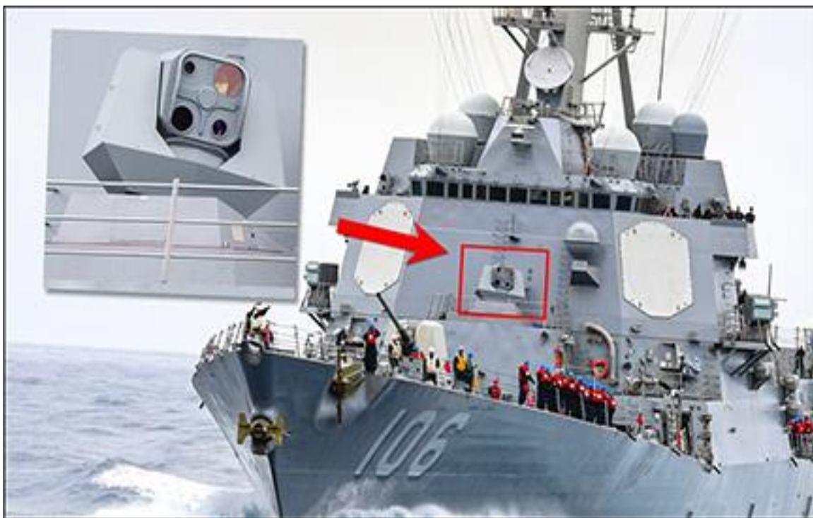
Figure 10. Reported ODIN System on USS Stockdale
