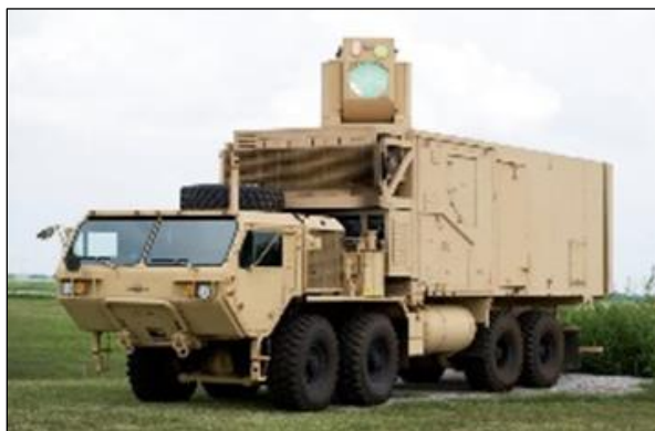
Figure 8. High Energy Laser Mobile Test Truck (HELMTT)
