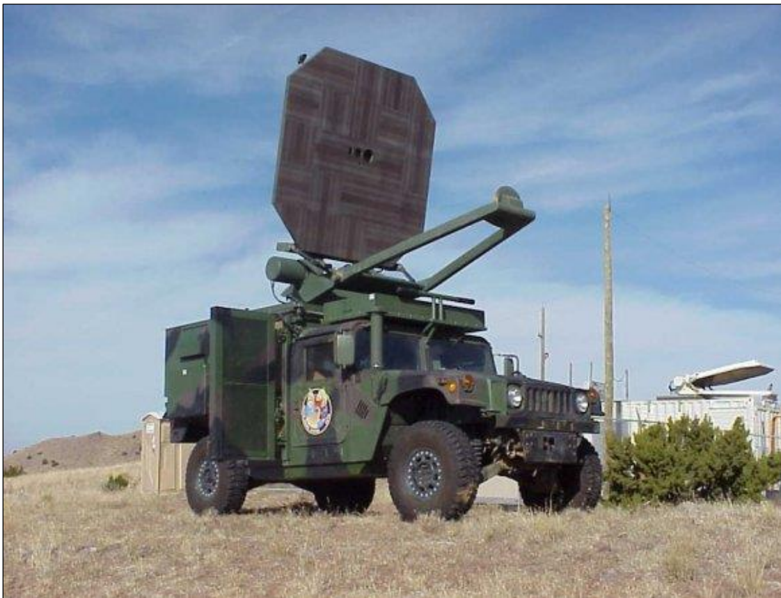
Figure 3. Prototype Army Active Denial System (ADS)
