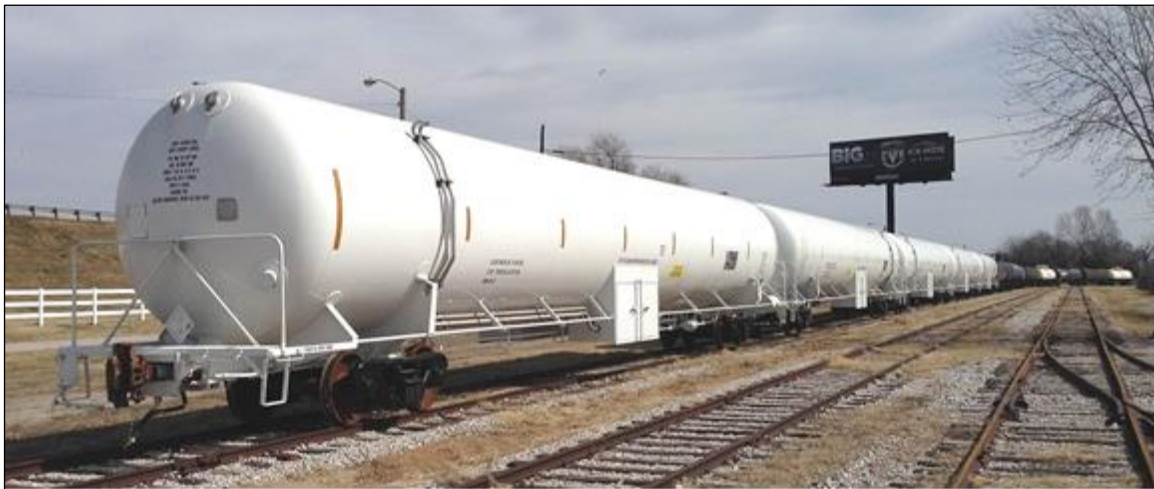
Figure 2. Insulated Rail Tank Cars Proposed for LNG
