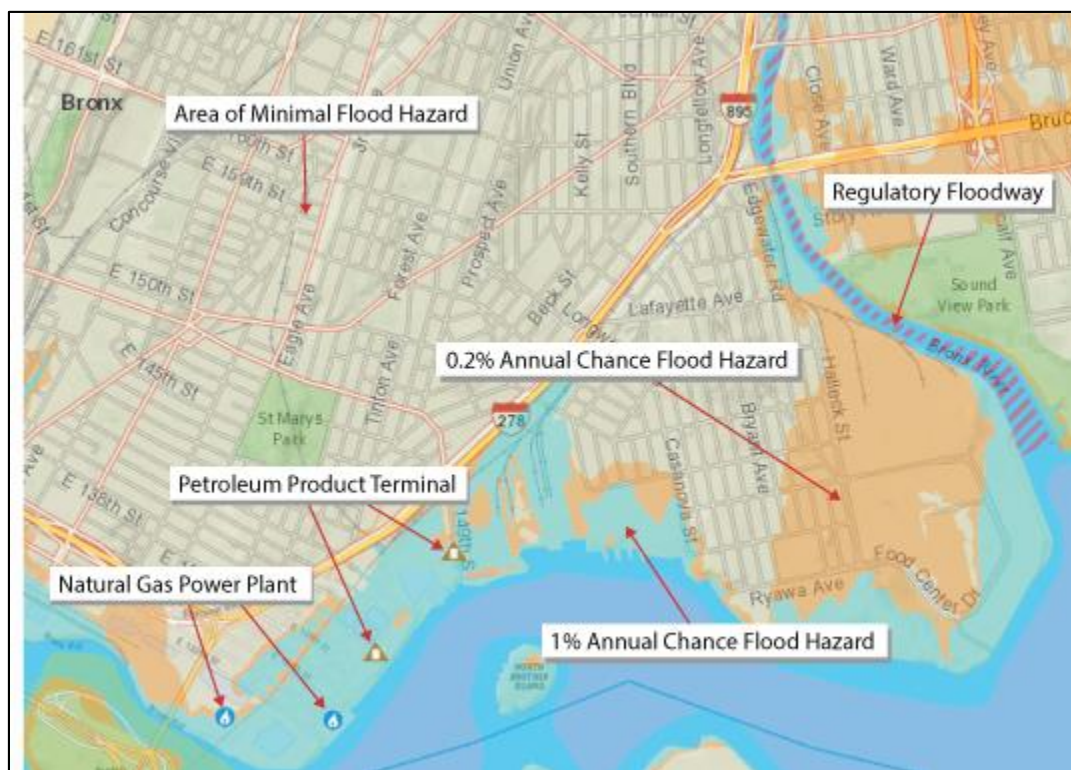
Figure B-2. Example Flood Vulnerability Assessment Map
