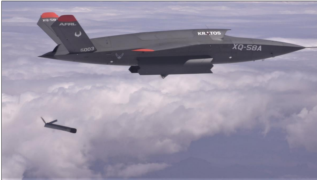
Figure 6. Valkyrie UAS Deploys ALTIUS-600 Small UAS
