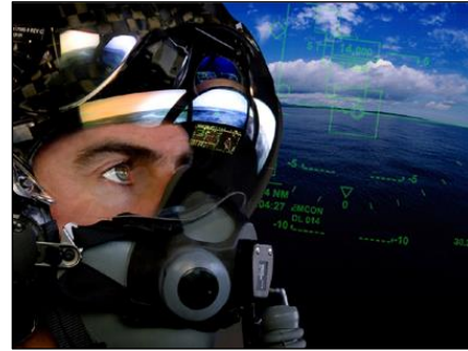
Figure 4. F-35 Helmet Mounted Display
